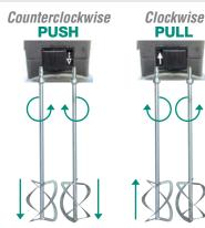
**Counterclockwise** rotation pushes material from the top to the bottom, reducing splashing when mixing low-viscosity materials such as paint, glue, filler and leveling compounds.
